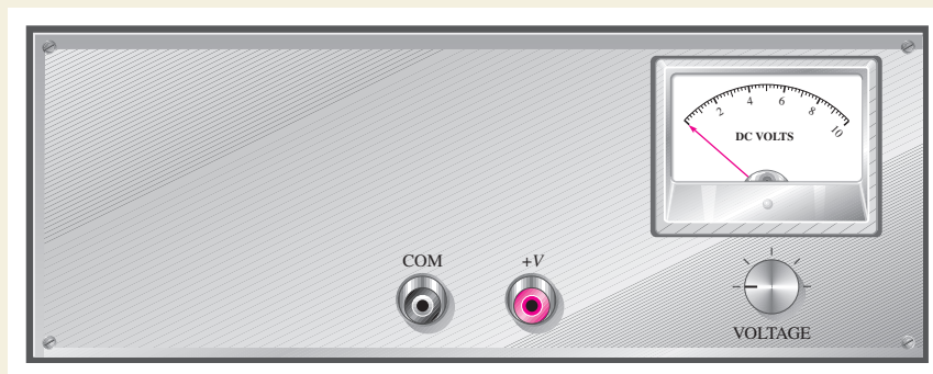
▲ FIGURE 49 Front panel view of a rack-mounted power supply.
